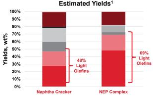
■Ethylene ■ Propylene ■ Crude C4s ■ BTX ■ Pygas ■ Fuel Oil ■ Fuel Gas ■ Hydrogen Both cases processing 3600 kMTA of HC LN NEP complex tuned to E:P=2.4
